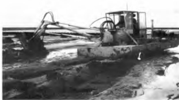
Fig. 13. Mechanization "Floating" excavator in low sedimentation field.
